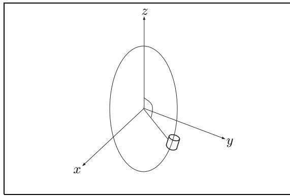
$$\begin{aligned} E' &= \frac{1}{2}mR^2\dot{\theta}^2 + V'(\theta) \\ V'(\theta) &:= -\frac{1}{2}mR^2\omega^2 \sin^2 \theta - mgR \cos \theta. \end{aligned} \quad (21)$$
